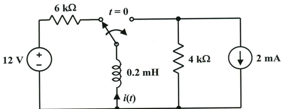
Assuming DC steady for  $t=0^-$ ,  $i(0) = -\frac{12V}{6k\Omega} = -2mA$
